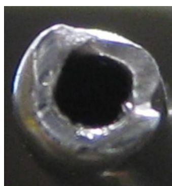
1/16" stainless steel tubing cut well. Notice the round hole.
