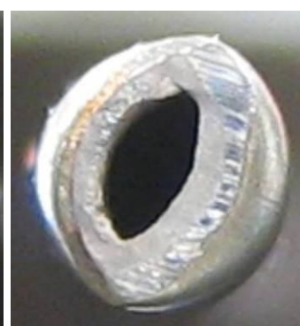
In this cut the hole is smashed into an oval. Ferrules may not even fit onto this tubing.
